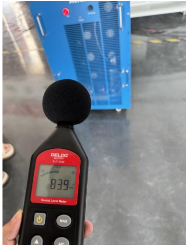
Sound level 84db fans in full operation. distance 1.5 meter
